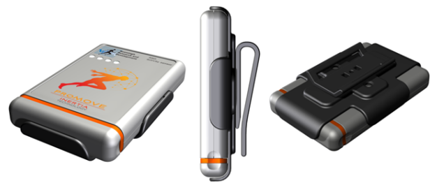
Figure 3: ProMove-3D node top view with clip holder (left), side view with belt clip (middle) and bottom view with elastic band clip (right).
